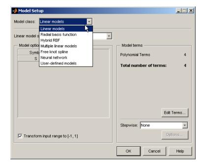
In the **Model class** drop-down menu is a list of available models. This list contains the same models that you would find in the global model setup of a one-stage model. Note the number of inputs changes which models are available. A local model with only one input can access all the models.
