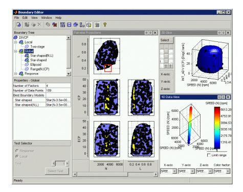
In this editor, you can construct boundary models from your data. Boundary models are nonparametric surfaces you can use as a visual aid to understanding complex operating envelopes. You can use boundaries to guide modeling and constrain optimizations.
