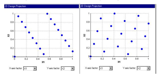
The preceding example shows the different properties of a poor lattice (left) and a good lattice (right), with a similar number of points. The poorly chosen prime number produces highly visible planes and does not cover the space well.
