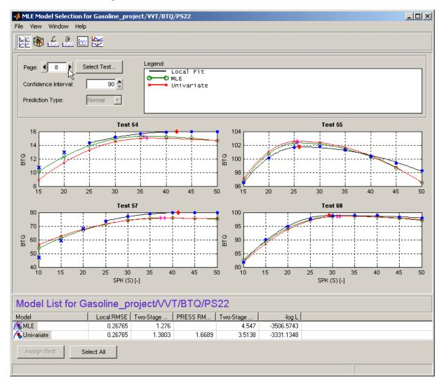
The tests view shows the data being modeled (blue dots) and models that have been fitted to this data. The black line shows the local model that has been fitted to each test separately. The green line and red lines in this case show an MLE two-stage model and the Univariate two-stage model: you can see the local model curves reconstructed using response feature values taken from the global models, and compare the fits.
