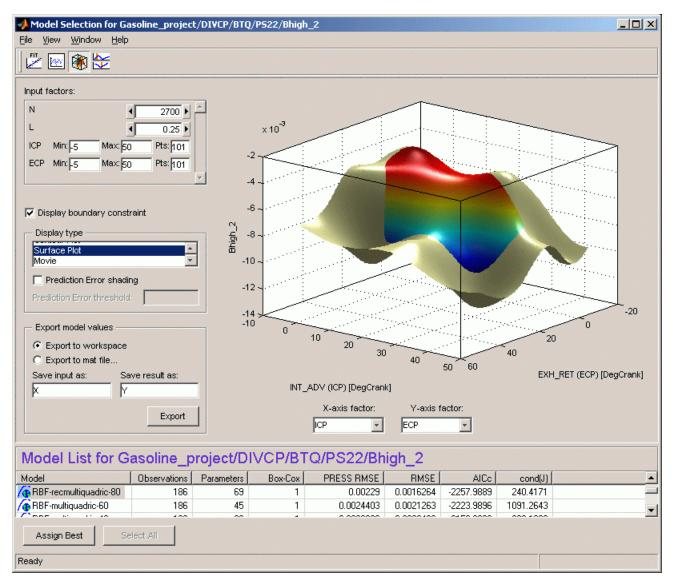
The default view is a 3-D plot of the model surface, as in the example. This model has five dependent factors; you can see these in the controls at the top left (there is a scroll bar as only four can be seen at once at this size of window).
