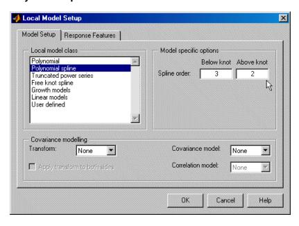
A spline is a piecewise polynomial, where different sections of polynomial are fitted smoothly together. The location of each break is called a knot. Polynomial splines are essential for modeling torque/spark curves.
