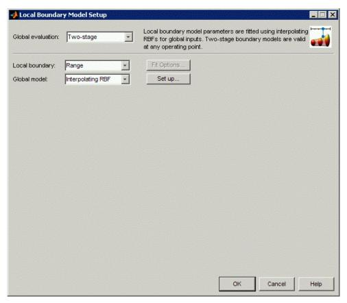
2 You can select Range or Ellipsoid for the Local Boundary (to fit to the local inputs).
