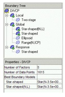
In this example, the root node (DIVCP) is selected—the icon is outlined. Look at the **Properties** pane to see which leaf node (or nodes) you have included in the set of best boundary models for the selected node—in this case, it is Star-shaped (all inputs) and the Star-shaped (N,L) global nodes. The icons in the rest of the tree show the path of combined nodes.
