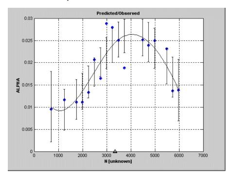
You can fit more complicated curves using splines, so they can be useful for the factor you expect to behave in the most complex way. This allows you to model detailed fluctuations in the response for one factor, while simpler models are sufficient to describe the other factors.
