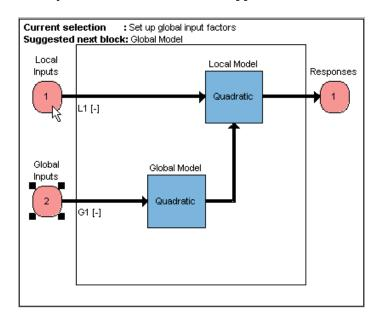
This example is a two-stage model. All test plan nodes show this view with a block diagram of the test plan. The diagram provides a graphical interface so you can set up inputs and set up models by double-clicking the blocks in the test plan diagram. You can also use the **Test Plan** menu.
