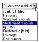
The preceding is an example drop-down menu on the scatter plot for changing x and y factors. In this case <code>spark</code> is the local input factor and <code>torque</code> is the response. The local inputs, the response, and the predicted response are always available in these menus. The observation number is also always available.
