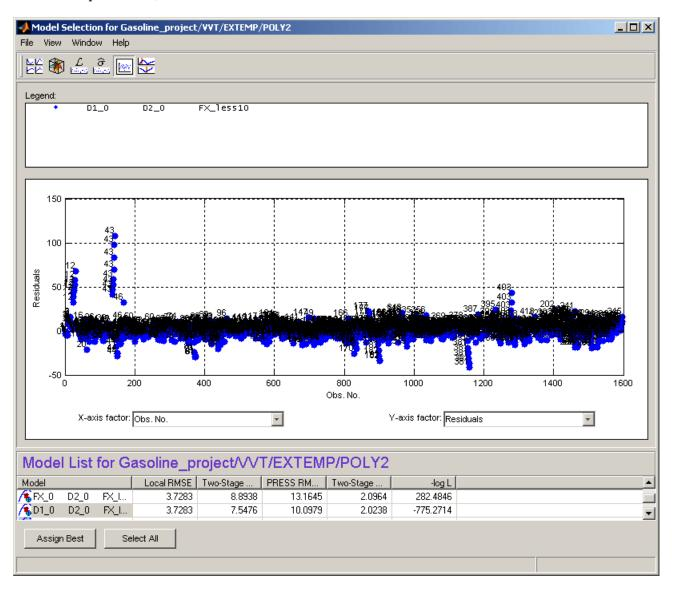
This view allows several models to be displayed simultaneously; click the **Select All** button at the bottom of the window or, in the model list view, **Shift**+click or **Ctrl**+click to select the models for display.
