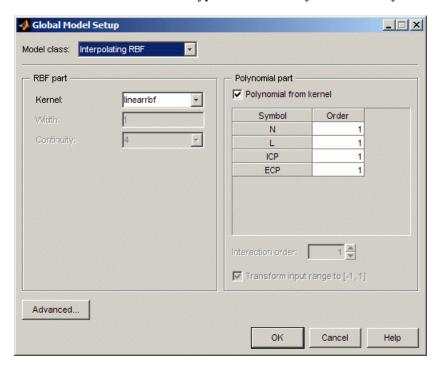
The **Kernel** drop-down menu offers the same options as for normal RBF. The **Width** and **Continuity** parameters are only enabled for specific kernels.
