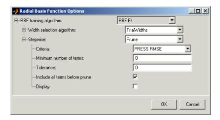
All the settings under Width selection algorithm are for fine-tuning the RBF model. See "Tips for Modeling with Radial Basis Functions" on page 7-22 for guidelines, and details on specific parameters for different algorithms can be found in "Radial Basis Functions for Model Building" on page 7-2.
