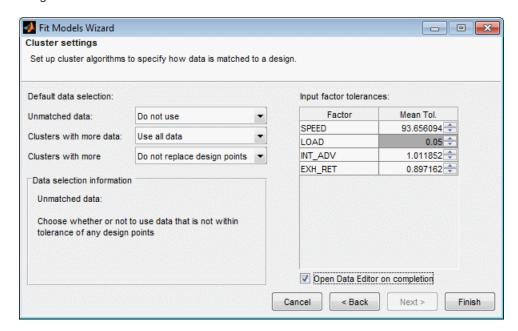
The choices you make in the **Default data selection** options determine how the cluster algorithm is first run to select matching data and design points. This only affects the status of the check boxes for data and design points when you first see the Design Match view in the Data Editor. You can always alter the results of this later in the Design Match list, where you can manually select the data and design points you want to use.
