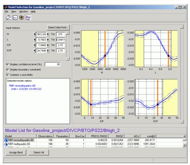
The number of plots is the same as the number of input factors to the model. The plot in S shows the value of the model for a range of values of S while the other input factors are held constant. Their values are displayed in the controls at the top left, and are indicated on the plots by the vertical orange bars.
