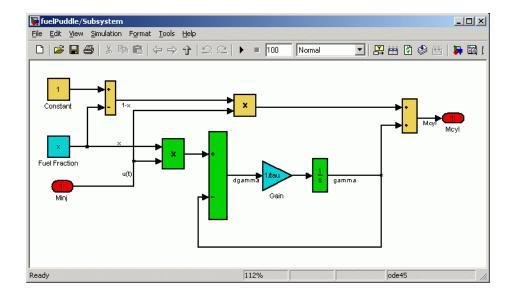
The block labels are not important. The model returns a single scalar output (here labeled "Mcyl").
