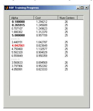
This is an example progress dialog box of a Tree Regression RBF model fitting in progress. Here you can see each trial value of alpha with its calculated cost and the best number of centers with that
