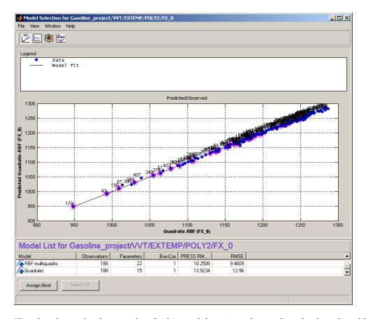
The plot shows the data used to fit this model, against the predicted values found by evaluating the model at these data points. The straight black line is the plot of y=x. If the model fitted the data exactly, all the blue points would lie on this line. The error bars show the 95% confidence interval of the model fit.
