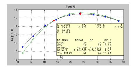
Here you see the values of the global variables for this test and some diagnostic statistics describing the model fit. Also displayed are the values (for this test) of the response features used to build this two-stage model and the two-stage model's estimation of these response features.
