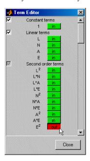
**Interaction**: You can choose the interaction level on both linear model subclasses (polynomial and hybrid spline). The maximum interaction level is the same as the polynomial order (for example, three for cubics).
