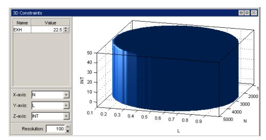
A 3D display to show the shape of this example constraint in the Design Editor can be seen below.
